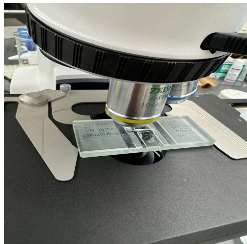
Figure 3. Hemocytometer and microscope, using 10x magnification
