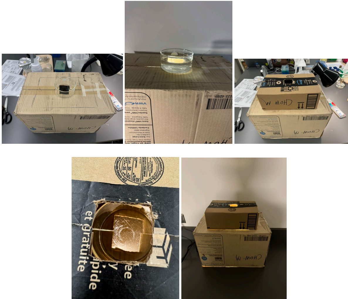
Figure 4-9, Setting up cardboard for lux measurement. (Top Left): I cut a hole in the center of the large box that is smaller than the glass container, so light can go through it. (Top Center): light penetrates the glass container and dH 2 O. (Top Right): setting another box to go on top of the larger box, the phone's camera would be set to align with the hole. (Bottom Left): top view of the whole system. (Bottom Right): another angle for the system (the phone is not in the picture yet)
