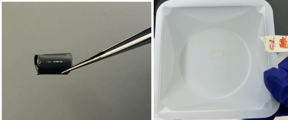
Figure 6: After day 7, it was noticed that white residue was built up on the bottom of the straw segment (left image). After day 10, (right image) it was noticed that there was shiny residue left on the bottom of the weigh boat. Specifically, for the acidic pH the residue had a pink tinge which was also the colour of the solution.
