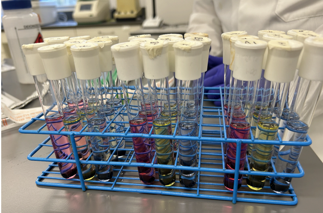
Figure 2: Test tubes containing PLA straw segments submerged in buffer solutions of varying pH (pH 4, 7, and 10) on the first day of the experiment. The color differences in the solutions represent distinct pH conditions.
