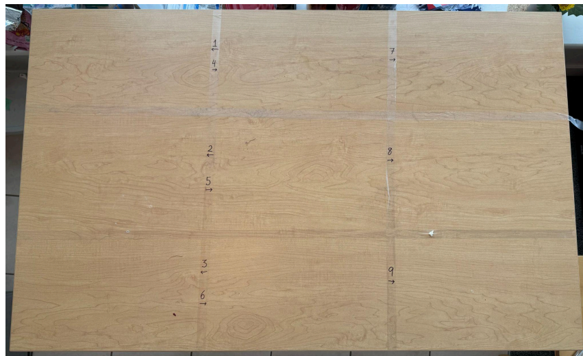
Figure 1. UBC dorm kitchen table divided into its nine even quadrants. Treatments were assigned to quadrants via a random number generator. The numbers on the tape indicate the quadrant number and the arrows indicate whether it is to the left or right of the tape border.
