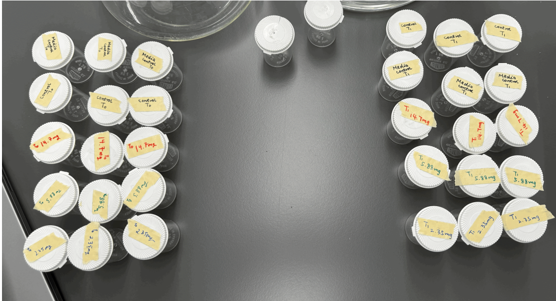
Figure 2: Image of all the vials created before they were filled with the corresponding solutions. Each treatment/control group was made of T_0 and T_f groups, made in triplicates; vials on the left were measured before incubation, and the matching vials on the right were measured after 3 hours incubation at 30^\circ\text{C} .
