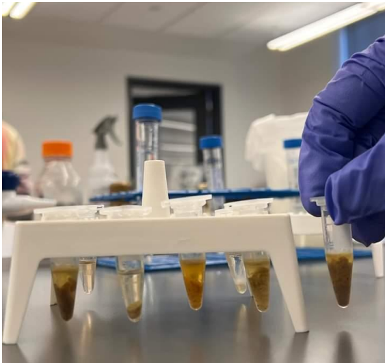
Figure 2: DNA isolation samples following initial centrifugation. Following the initial centrifugation, different levels of softening and sample volume impacted supernatant extraction.
