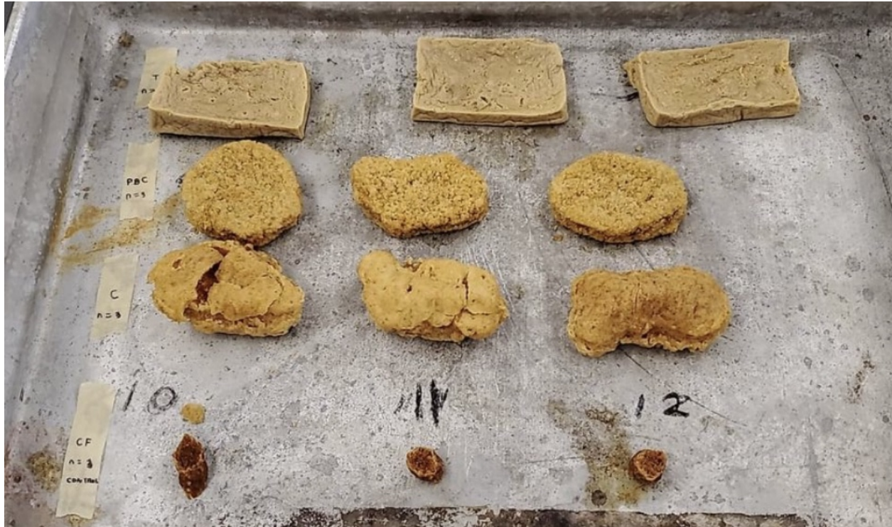
Figure 5. The 4 groups of samples after oven-drying at 90 degrees C in the initial procedure.
