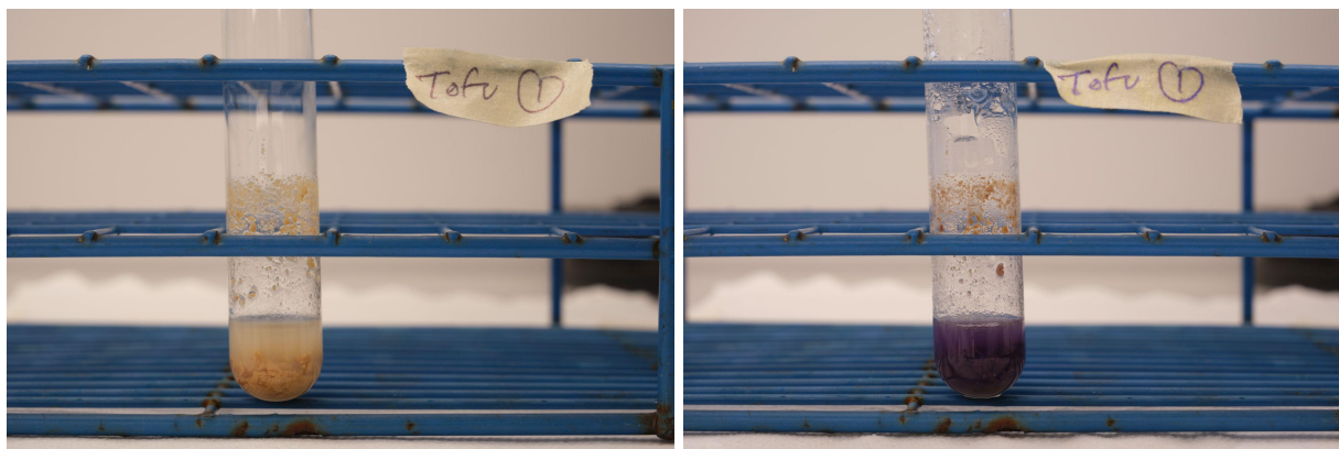
Figure 2. Before and after photos of tofu-ninhydrin solution after 20 minutes of water bath heating at 90 degrees Celsius.
