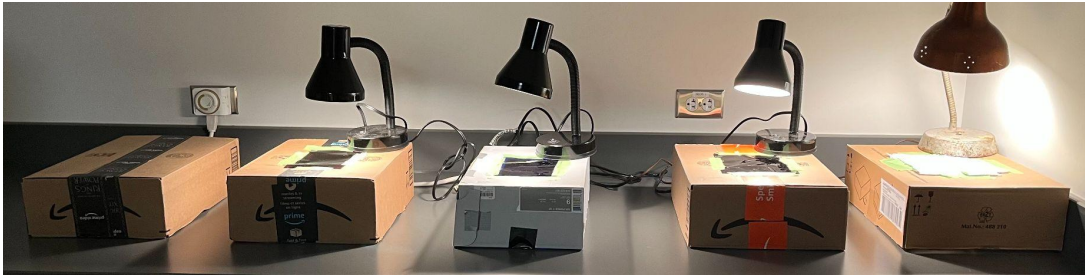
Figure 1. The set up of the five treatment groups from left to right: no light, red light, blue light, green light, and white light. All treatment groups were kept at room temperature. The box without a lamp represents the dark control group. All lamps are situated in the top right corner of each box to ensure a similar angle of light exposure to all seeds. A light intensity of 35 \pm 10 Lux was held constant for all groups.
