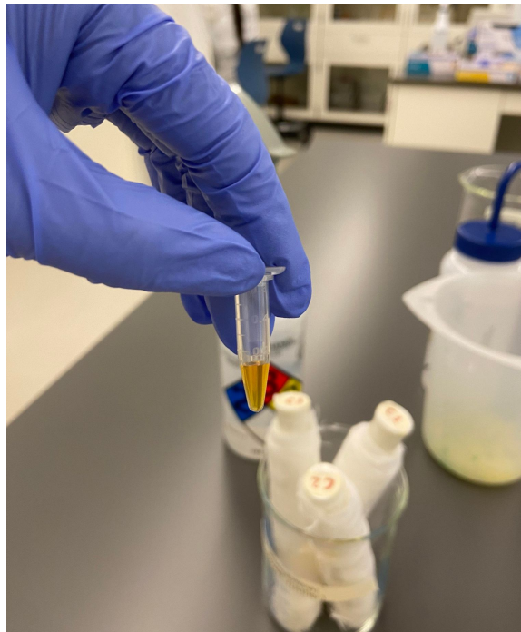
Figure 7. An example of a sampling tube containing 10 uL of potassium iodide fixative plus 100 uL of a C. reinhardtii sample.
