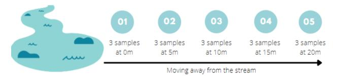
**Figure 1. Overview of soil sample collection method.** Blue circles display the transect number; transects are located every 5 m moving away from the stream; 3 samples were taken at each transect; each sample was taken around 10cm below the surface.
