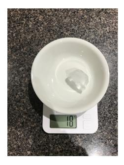
**Figure 1.** Displays the weighing scale as part of the experimental set-up. The AccuChef weighing scale was used to measure the initial and final weights of the ice cubes. This instrument provides readings in grams (g) to whole number digits. A ceramic plate was placed on the scale and tared to allow for a reading of the ice cube prior to and following exposure to a melting agent.
