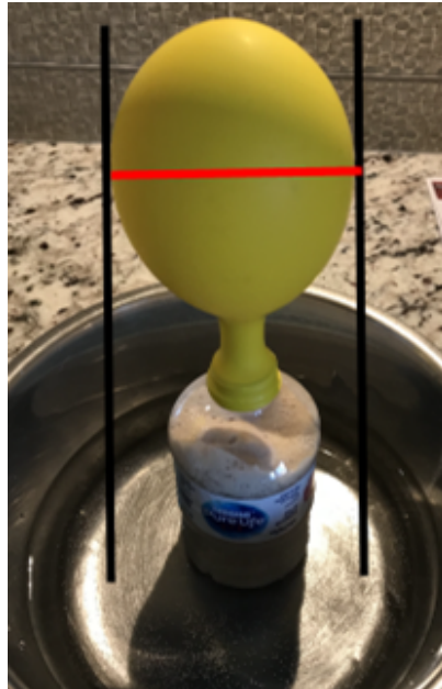
Figure 1: This figure shows how the diameter of the spherical part of the balloon was measured. The black and red lines depict rulers. The red line between the two black lines was how the diameter of the balloon was measured. This figure also depicts the cylindrical base or neck of the balloon.
