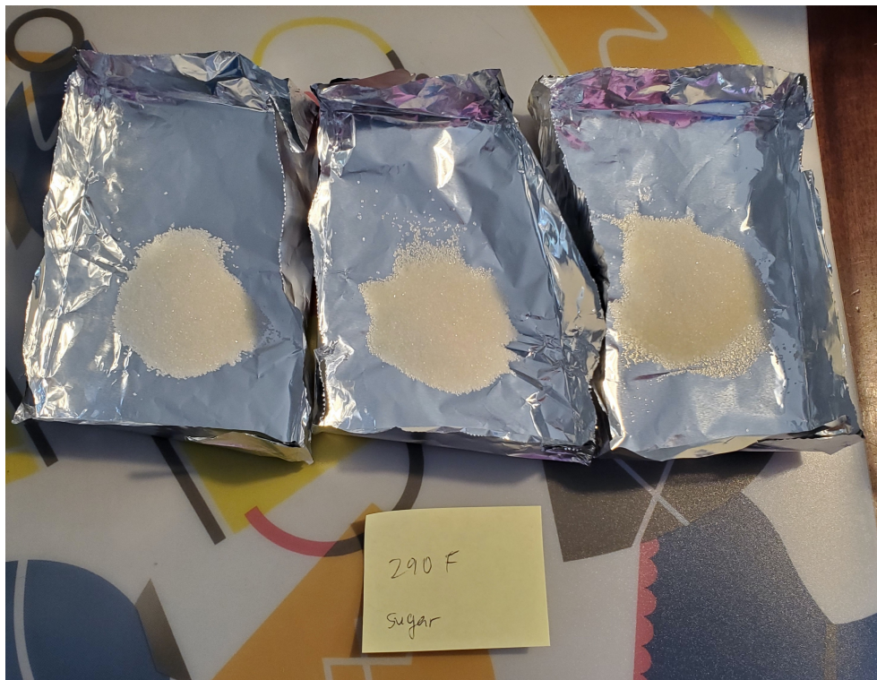
Figure 1: 3 replicates of sugar in the oven at 290F dial temperature. The left sugar sample did not melt. The sugar samples in the middle and on the right melted along the edges of the sugar pile.
