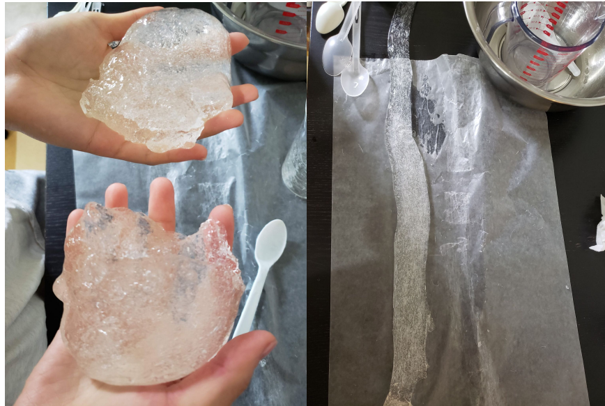
Figure 1. Left: Slime made with 1 \frac{1}{4} tsp borax breaking with no stretch. Right: Slime made with 1 tsp being stretched. Gloves were removed to stretch the slime since the slime kept sticking to the gloves, making it difficult to manipulate properly.
