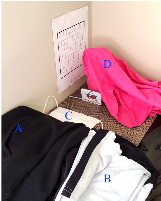
Figure 1: Experimental set-up to test the effectiveness of fabrics at reducing the spread of respiratory infections. (A) 80/20 cotton-polyester blend clothing item (n=8). (B) 100% polyester clothing item (n=8). (C) Disposable mask (n=8). (D) 100% cotton clothing item (n=8)
