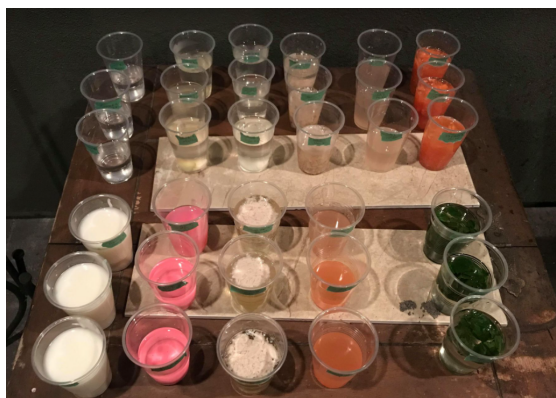
Figure 1. The experimental setup, with 3 replicates of each test ingredient placed in white vinegar. Each cup was labelled with the test ingredient and replicate number. All the ingredients were left in the cups for 30 minutes after mixing with white vinegar.
