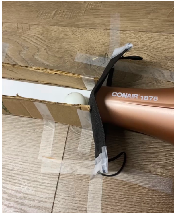
Figure 1. Picture of the start of the cardboard path showing the optimal placement and set up of hair dryer, mask and ping pong ball.
