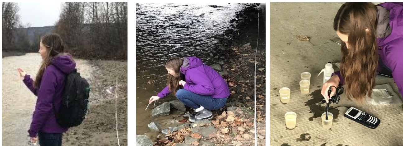
Figure 2. Images of air temperature, water temperature, and dissolved oxygen levels being measured at Baker Creek in Quesnel, British Columbia.
