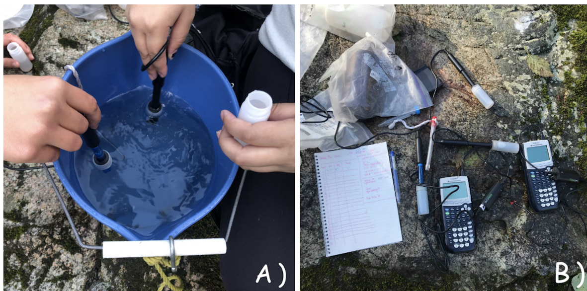
Figure 2. 2a demonstrates the methodology for obtaining sample measurements using the Vernier pH sensor and DO probe. 2b displays the equipment utilized during measuring, including the TI-84 calculators which contained programs necessary for DO and pH measurements.
