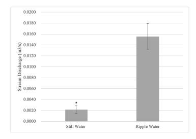
Figure 3. Mean stream discharge (m<sup>3</sup>/s) at still water (left) and ripple-water sites (right) (n=6). Error bars represent 95% confidence intervals (0.34 at still water site, 0.002 at ripple site), where  $p \le 0.05$ . The standard deviations for still water and ripple sites are 0.00215 and 0.00295, respectively. The t-value is 10.67 and p-value is <0.00001.
