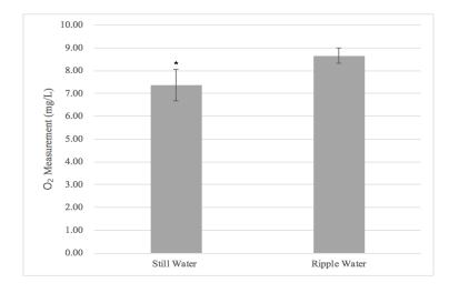
Figure 2. Mean oxygen levels (mg/L) at still water (left) and ripple-water sites (right) (n=6). Error bars represent 95% confidence intervals (0.68 at still water site, 0.000686 at ripple sites), where  $p \le 0.05$ . The standard deviations for still water and ripple sites are 0.86 and 0.42, respectively. The t-value is 3.24 and p-value is 0.0089.
