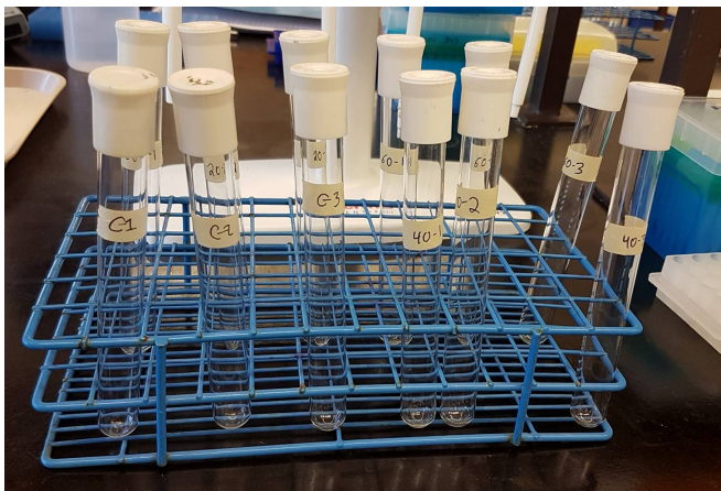
Fig. 2 Test tube rack holding the replicates of each treatment labelled as treatment-replicate (ie.- Replicate 1 for 0% fertilizer concentration is seen as C-1).
