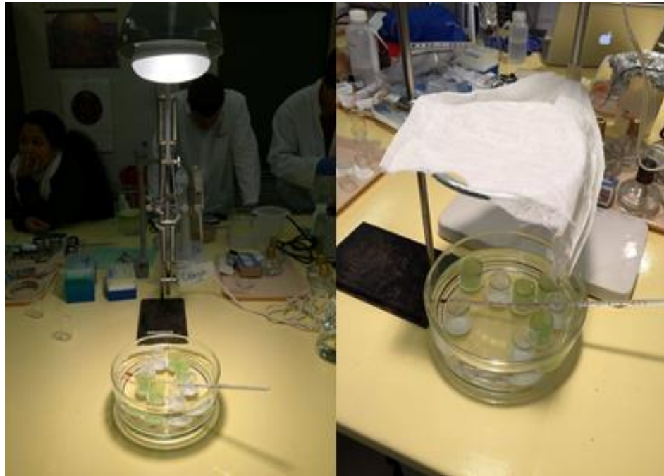
Figure 2. Left: One of the treatment set-ups at 5000 lux with replicate and control pairs placed in the water baths. Right: An image of the folded mesh cloth between the lamp and the water bath needed to obtain 1000 lux.
