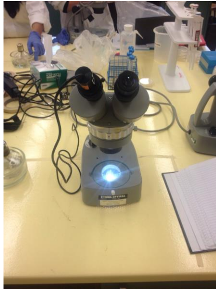
Figure 2. Kyowa dissecting microscope with the DinoXcope attachment.
