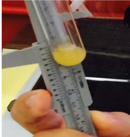
Figure 4. Measuring the height of bubble formation using a caliper
