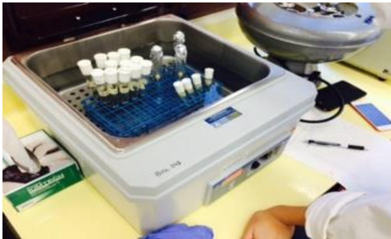
Figure 3. The setup of the respirometers inside the water bath at 30°C
