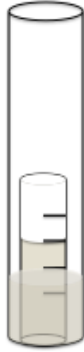
Figure 3. Example setup of respirometer tube. Figure shows \text{CO}_2 produced at top of small inner tube and yeast-sugar solution being pushed out of the bottom. Markings represent 0.5 \mu\text{L} increments.
