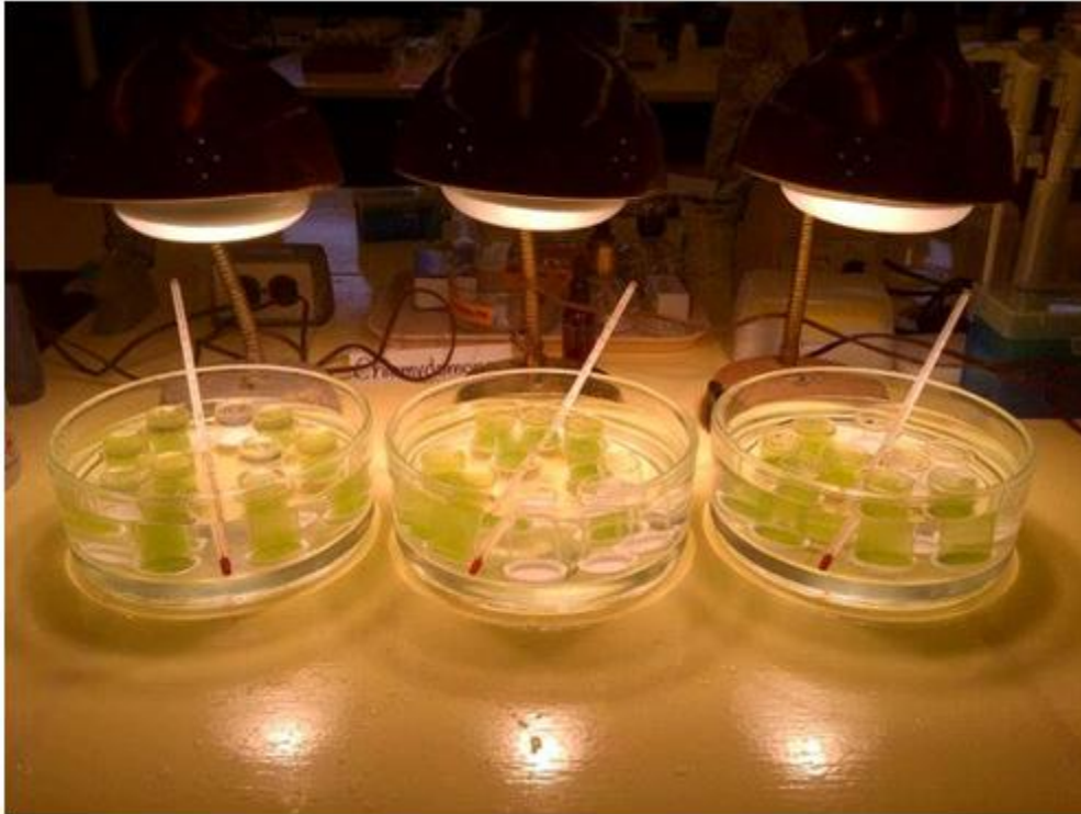
Figure 5. Our experimental set-up. Three C. reinhardtii mutant, three wild type, and three procedural control replicates in each water bath (temperatures from left to right: 15°C, 22°C, and 27°C) under 150W flood lamps.
