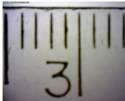
Figure 2. Sample image of ruler calibration under the dissecting microscope.
