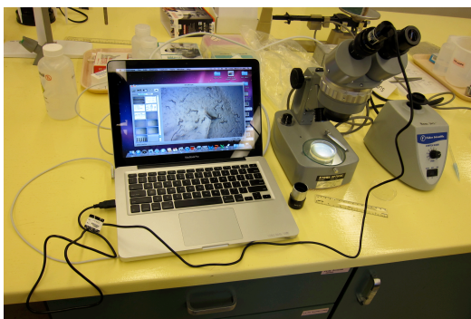
Figure 1. Image of dissecting microscope with Dinoxcope ocular camera set up at 17°C.
