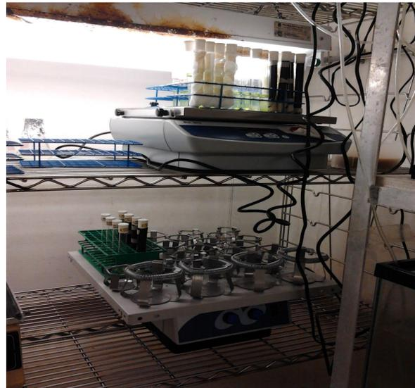
**Figure 2:** Experimental setup under separate light intensities in incubator. 5000 Lux samples on top shelf, 970 and 0 Lux on bottom shelf.
