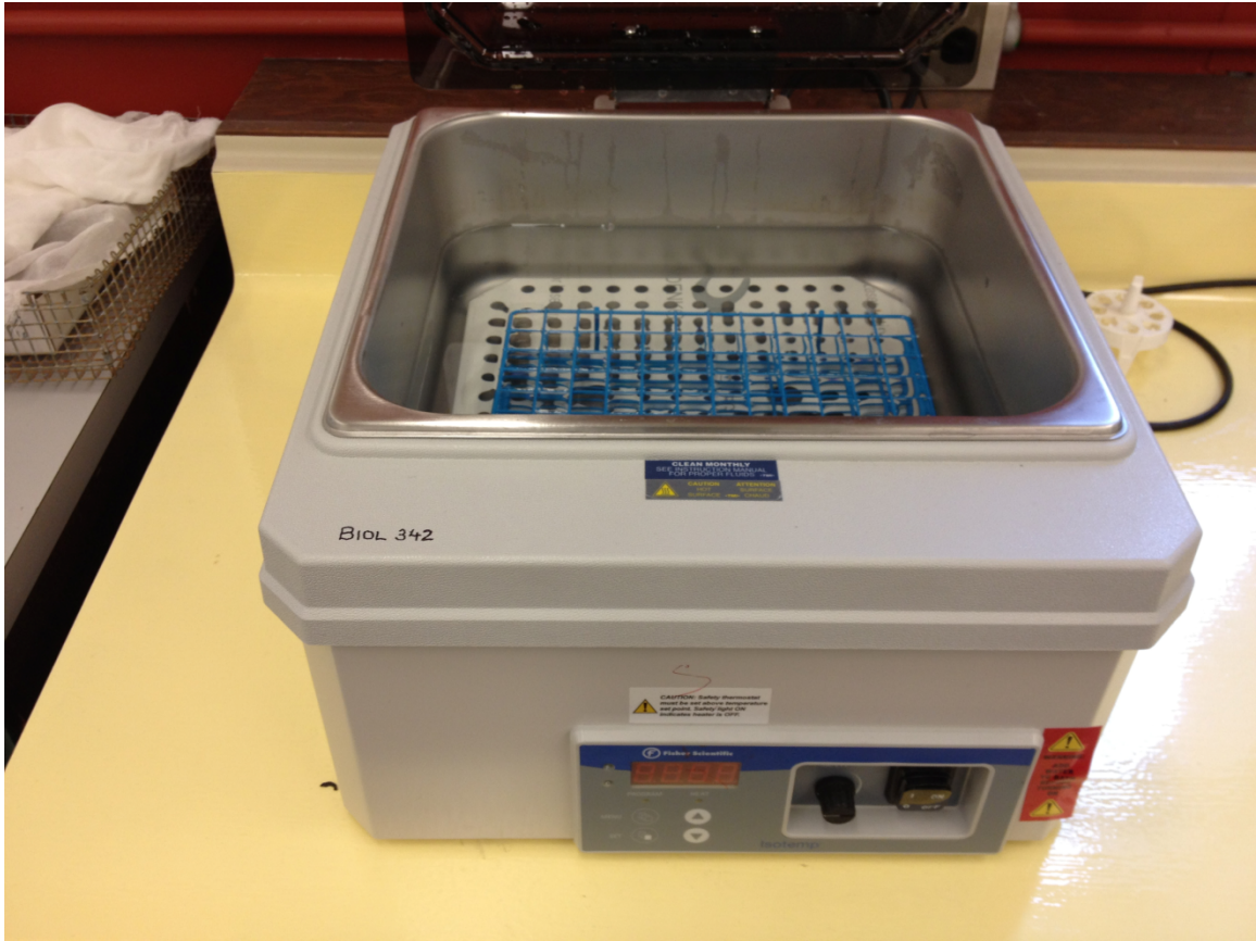
Figure 1: 30°C water-bath with test-tube tray set in water. Temperature is adjusted using knobs on bottom right, and lid is closed during incubation.
