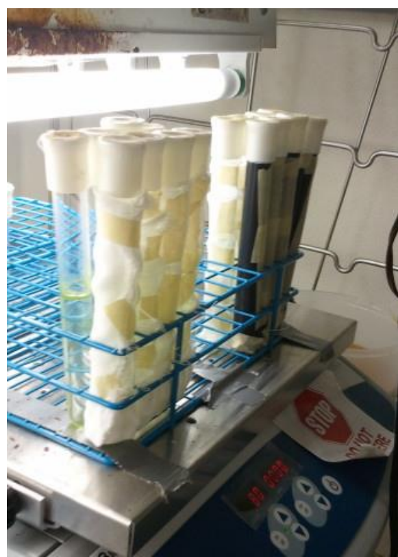
Figure 1 C. reinhardtii cells in their respective treatments test tubes on a shaker set at 80 rpm, inside the 17°C incubator. Cultures are under fluorescent light bulbs. Right: single layer of cheesecloth (5700 Lux); black plastic (0 Lux). Left: control, no filter (8020 Lux); four layers of cheesecloth (3180 Lux).
