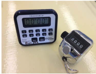
Figure 2: Stop watch and counter used to count cell densities and motility speeds.
