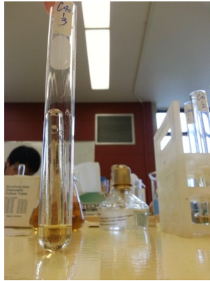
Figure 1. The setup of a respirometer with a small test tube filled with solution inverted inside a big test tube.
