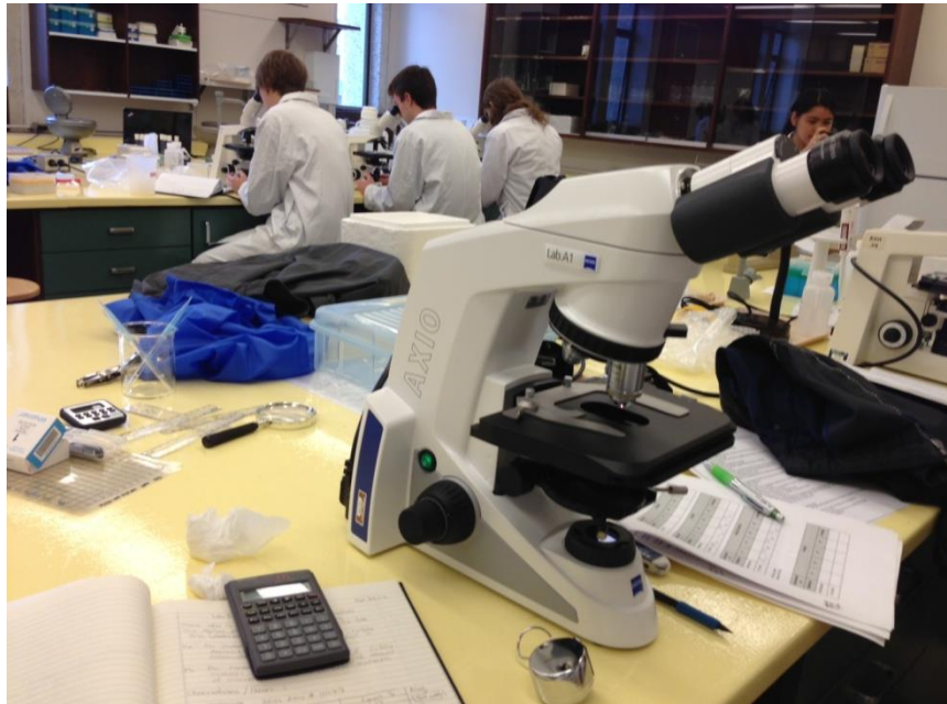
Figure 1: Cell counts were done through a Zeiss Axio microscope with the sample on a haemocytometer.
