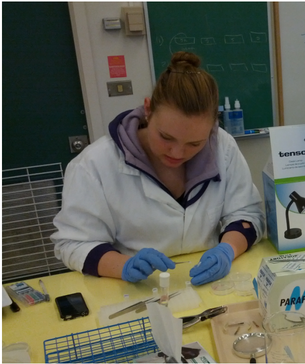
Figure 1. Preparation of the filter paper circles. In this figure, the filter paper circle is being placed into a centrifuge tube to soak.
