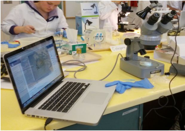
Figure 2. DinoXcope set up. The camera was placed in the eyepiece of the microscope and connected to a laptop.
