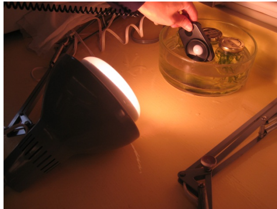
Figure 7. Trial 2. Measuring light intensity of the middle replicate using a Fisher Traceable® Dual-Range Light Meter of Treatment 2.
