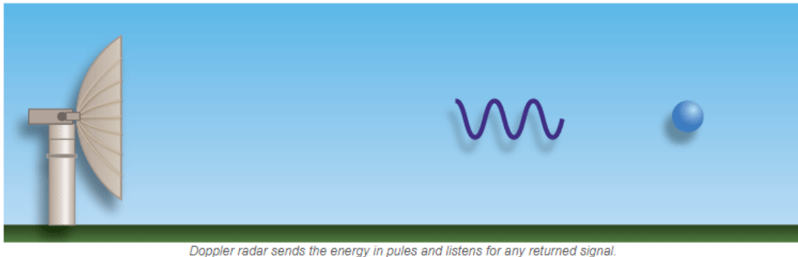
Figure 3. A weather radar emits a radio wave and waits for a return wave to determine the object. ( https://www.weather.gov/jetstream/how )
