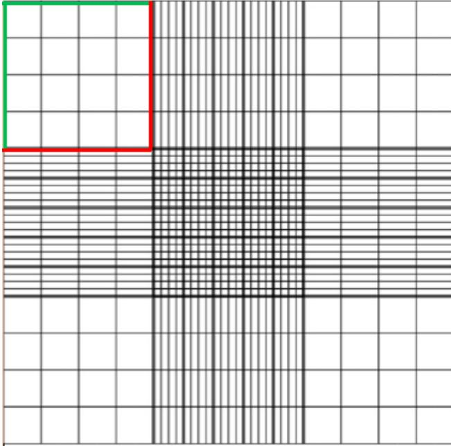
**Figure 2.** This hemocytometer grid demonstrates the standardized method of counting that was used. For cells on the edges of squares, only those on the edges marked in green were counted for each square. Adapted from “What is a hemocytometer?” by M. Jalan, 2019 (<https://www.scienceabc.com/pure-sciences/what-is-a-hemocytometer-calculation-counting-how-to-use.html>).
