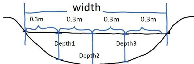
Figure 1. A cross-sectional illustration of a stream showing how measurements were performed to obtain stream discharge.
