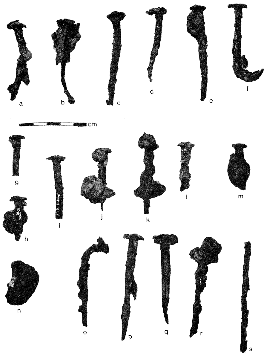
FIGURE 8. Nails and nail fragments: a , six penny rose head nail with flat point; b , c , eight penny rose head nails with uat points; d , six penny rose head nail with sharp point; e , eight penny rose head nail with sharp point; f , ten penny rose head hinge nail; g-n , rose head nail fragments; o , eight penny T-head brad; p , ten penny T-head brad; q , eight penny round-head, round shank nail; r , nail fragment; s , iron rod end.
