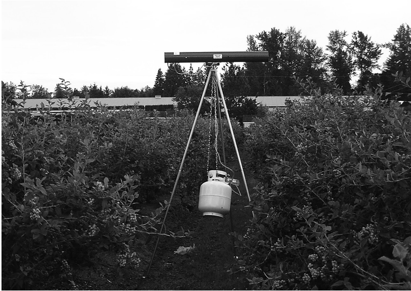
Figure 1. A triple-shot propane cannon. Photo courtesy of the BC Ministry of Agriculture.
