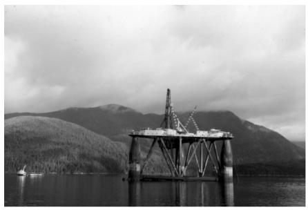
Figure 6. Sedoco 135F moored in Mooyah Bay, Nootka Sound, as seen from MV *Uchuck III*. The rig was occasionally towed into deep sheltered harbours to make repairs. The size of the rig is indicated by the barely visible Bell 205 helicopter perched on the right-hand leg. Photo by George B. McCandless.
