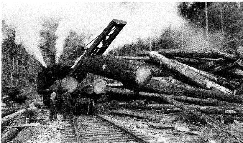
Logging Process, Yarding & Loading: Logging Crane “heeling” large pine log and about to swing it into car, 1940s. Special Collections, UBC Library, MacMillan Bloedel Limited Photograph Collection, Box 15, BC1930/131.
