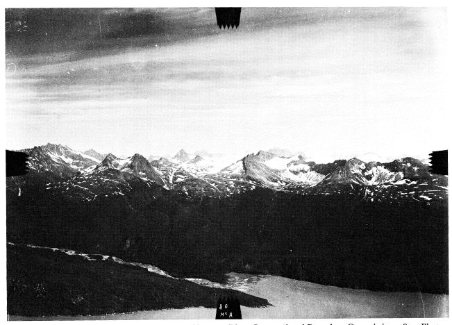
PLATE VII. Station Moore 139, mouth of the Skagway River. International Boundary Commission, 1894. Photo: J. J. McArthur (PA-37709). McArthur was the most experienced of Deville's phototopographers. This photograph is typical of the work of all the surveyors on the International Boundary Commission and forms part of a 360° panorama. It is evident that this photography is purely practical and has no existence other than to convey specific surveying information.
