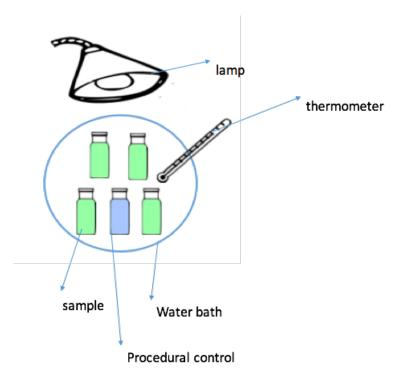
Figure 3. Setup of our samples in the water bath
