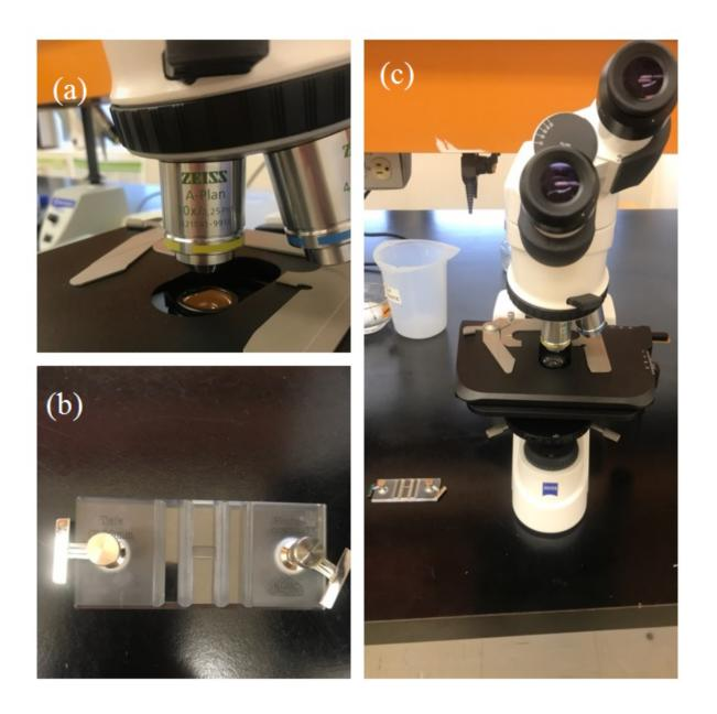
**Figure 1**. Set up to determine initial concentration of media. (a) is the magnification used to view cells. (b) is the specific haemocytometer (note: labeled) used to count cells. (c) is the Axiostar compound microscope used to view cells.
