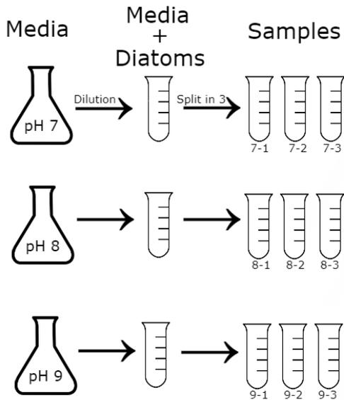
Figure 1. Showing the preparation of the 9 growth tube samples.
