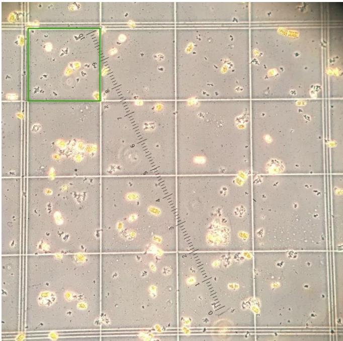
Figure 2. Direct view of a hemocytometer through a compound microscope lens (10x) showing the “green square” used for counting. *L. abbreviata* is shown under pH 7 conditions.
