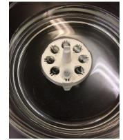
Figure 4. Microcentrifuge tubes with 1 mL of either mutant or wild-type *C. reinhardtii* were submersed in water baths set to the treatment temperatures (20°C, 25°C and 30°C) for 10 minutes prior to observation.
