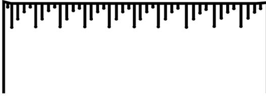
Figure 7. The staggered pattern of stitching around the rim makes the containers stronger and prevents tearing.
